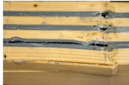
Fig 2b: Fiber buckling of both, timber and CFRP laminates, in the compressive zone.
