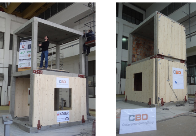
Fig. 3: CLT strengthening system developed in Slovenia
