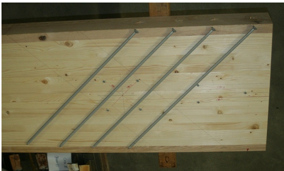
Fig. 1: Beam reinforced with SFS screws 13 mm x 800 mm (principal)
